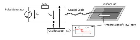
Figure 2: TDR sensor setup
