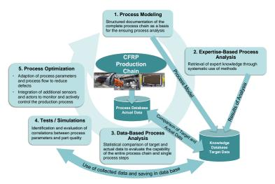
Figure 1: Methodical approach to model, analyze and optimize CFRP production processes
